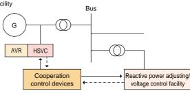
Cooperation control of HSVC and other reactive power adjusting/ voltage control facility.
